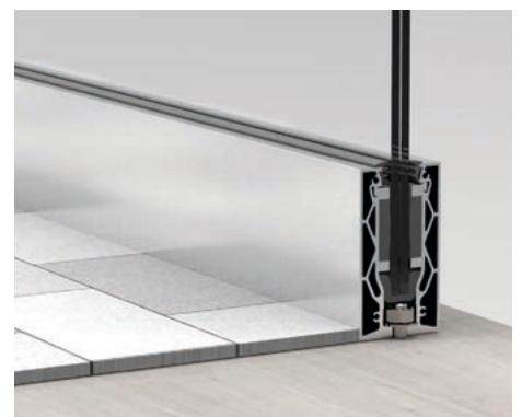
8. Fertiges System mit Bodenbelag completed system with flooring
